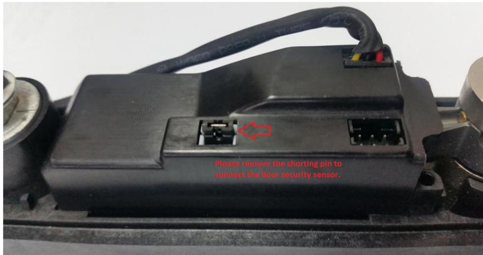
The closeup picture above shows how the jumper should be present if no door sensor is being used. The port on the right is where the cable is connected from the lock to the SP2+ sensor port as shown in the installation video (link provided above).
