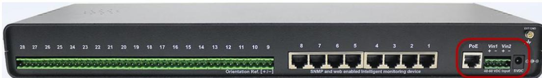
**DCW Units - sensorProbe8-X20 & X60 DCW** – The DCW power inputs are circled in the above image. The DCW internal power supply option is only available on the X20 and X60 units. The dual inputs can provide redundant power to the units when connecting two separate voltage sources. The DCW units support +/- 48VDC operating voltage.
