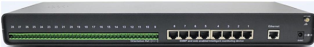
The rear view of the SP8-X20 shows the 20 dry contact inputs, the 8 intelligent sensor ports 1 through 8, the 10/100 Ethernet port, the 5VDC AC power input and the GND grounding stud.
