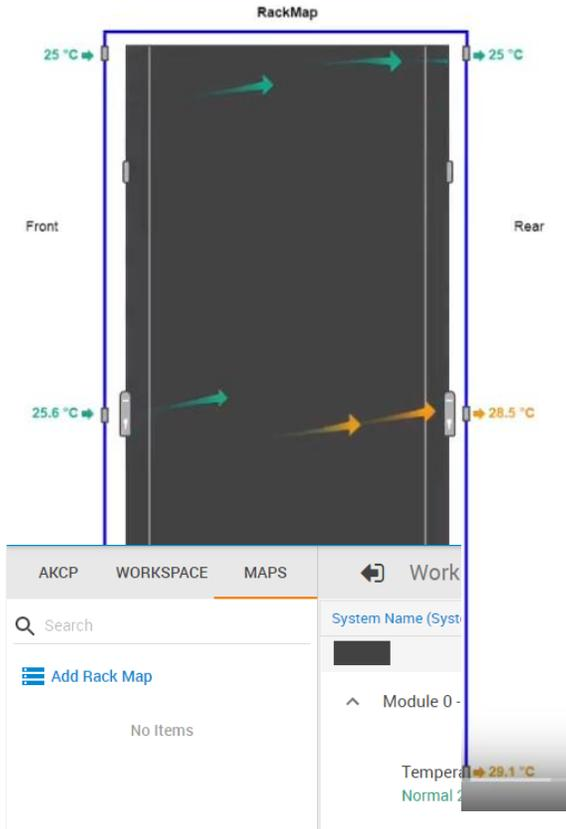
The Rack Map feature was originally (and still is) included in the AKCess Pro Server / AKCPro Server (HTML5) and has also been added to the SP+ units. You can add a Rack Map as a graphical representation of your server rack, and to display and record the temperature of the airflow within your server cabinets.
