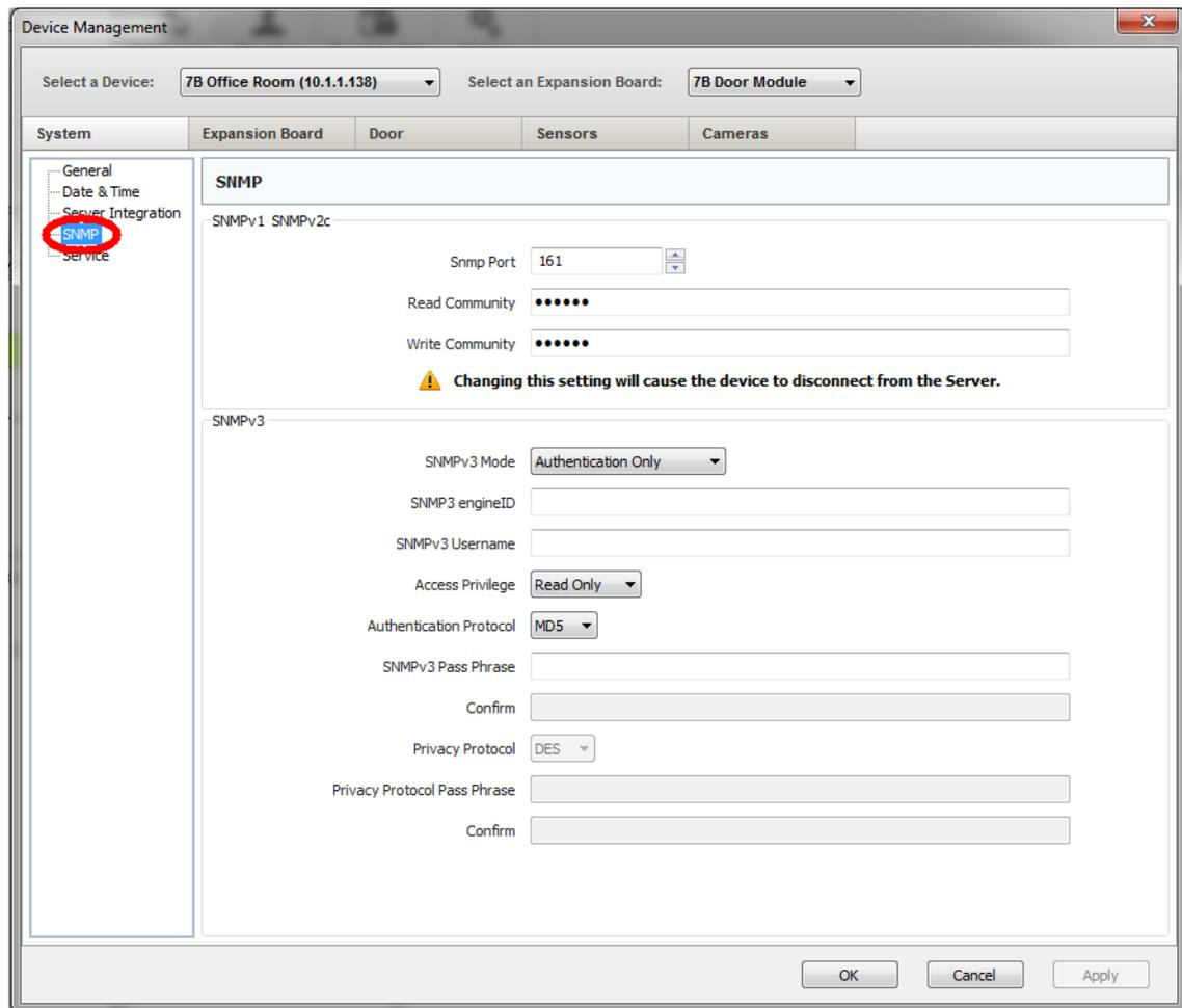
SNMP – Settings for SNMPv1, v2 and v3 including Read and Write Communities
