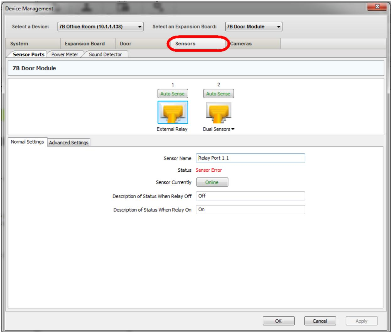
By clicking on the Sensors tab we can configure the sensors that are connected to the two RJ-45 sensor ports on the DCU. Please see each separate RJ-45 AKCP Intelligent Sensor user manual for specific information on each sensor.
