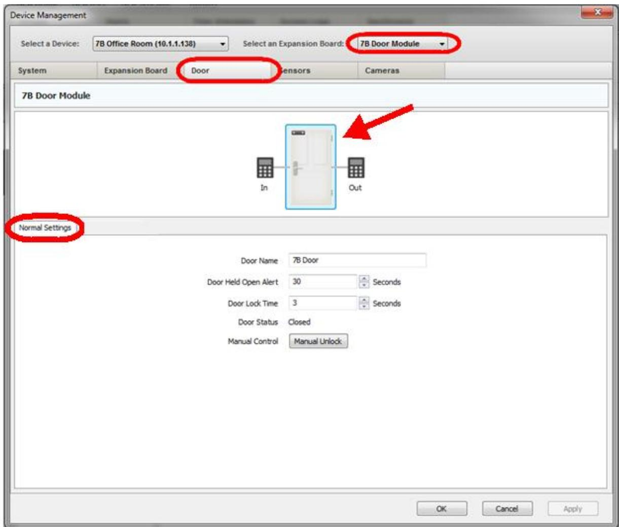
The Door tab is where we will setup the DCU to control the door lock, the card and finger print reader for the door. First we click on the door icon that the arrow in the screen shot above shows.
