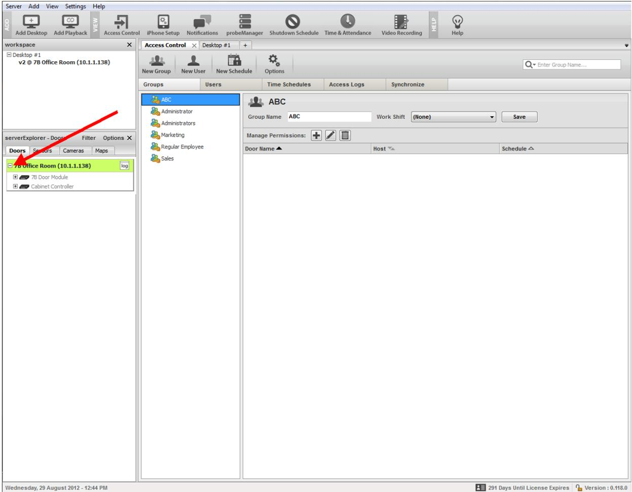
By clicking on the expand or the + icon in the serverExplorer we can now see our DCU unit and that the unit is online and connected successfully to our server. If there was a problem with the connection the color would be showing Red.
