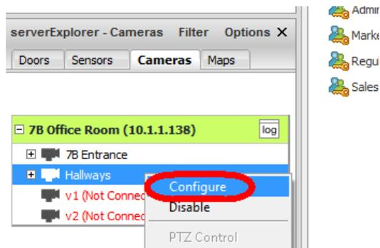
You can also open the camera configuration page by right mouse clicking on the cameras in the serverExplorer and clicking on Configure as shown in the screen shot above.
