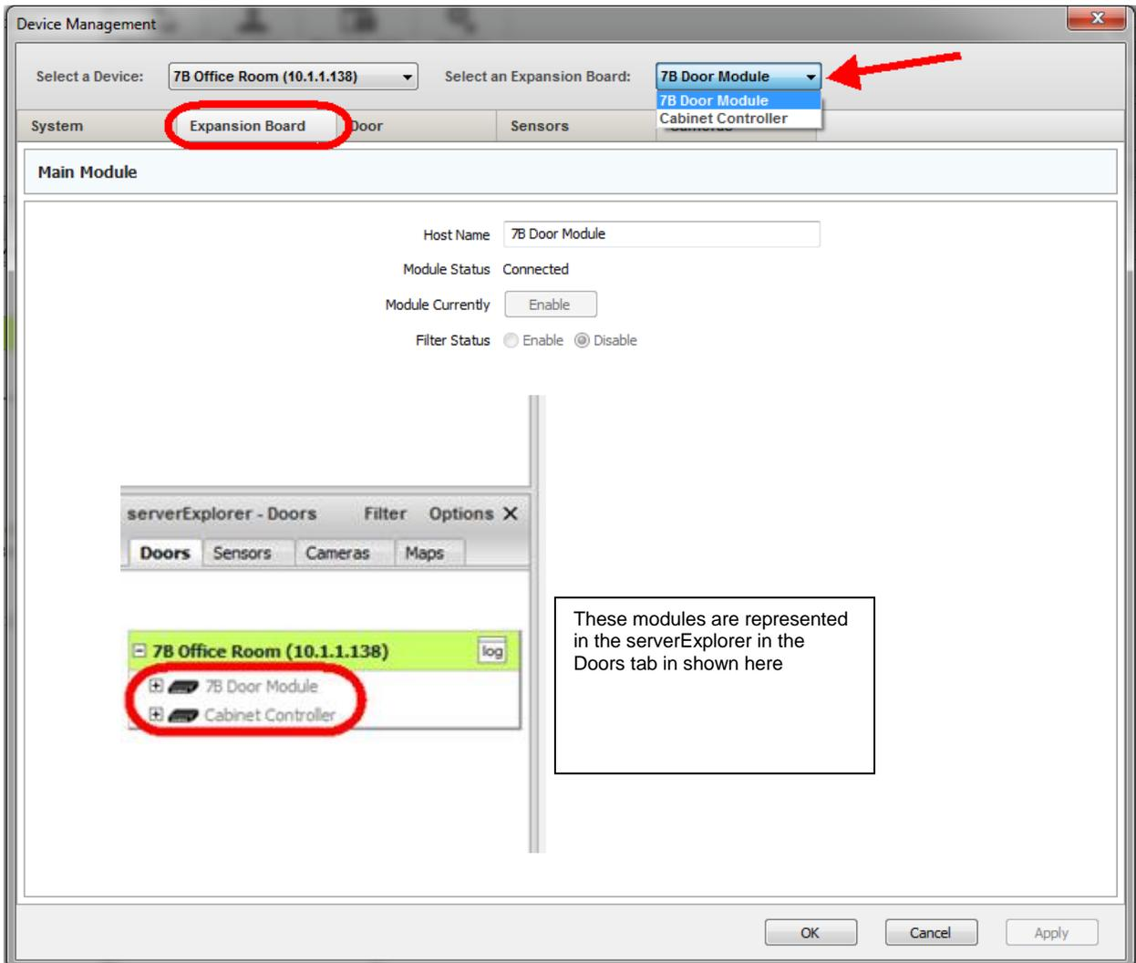
The Expansion Board tab is where we can check the status of the Main Door Controller Module , enable or disable additional CCU's (Cabinet Control Units) or additional Expansion Units such as an E-sensor8 Expansion unit.
