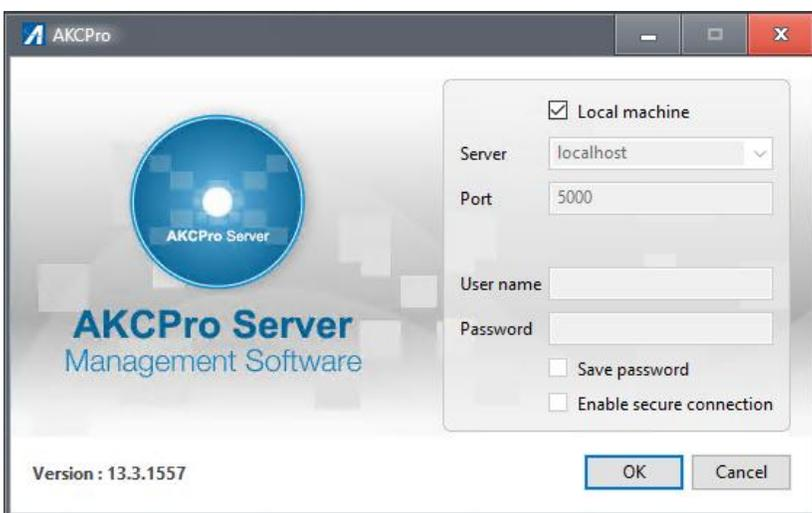
To log in to the locally installed server, you can just click the option **Local machine** and press OK; it will log you in without any password requirements. To ensure security, you'd have to make sure that access to your server's console is restricted.
